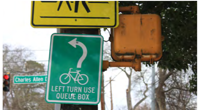
Signage directing bicyclists to use a queue box at a signalized intersection
